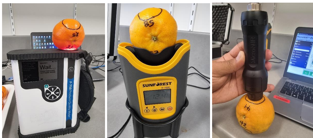
Figure 30. F-750 (left) SunForest (middle) and MicroNIR (right) devices (from Aryal, 2022 ).
