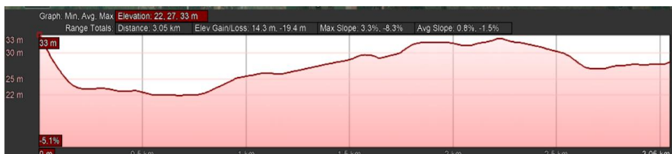
Figure 32. Example ground elevation profiles from GoogleEarth between sensor location and gateway location (packshed). The aerial position was 3 m higher than ground level for sensors, and 6 m higher for gateways.
