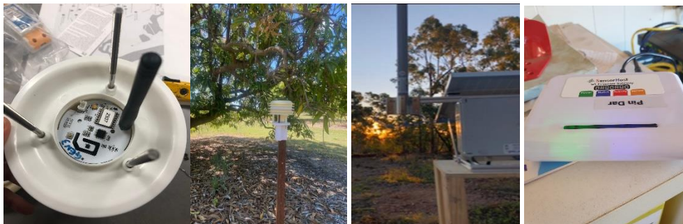
Figure 31. (a) SensorHost electronics board; (b) Stevenson screen mounted at 1.2 m height on a star picket; (c) repeater unit; (d) gateway.
