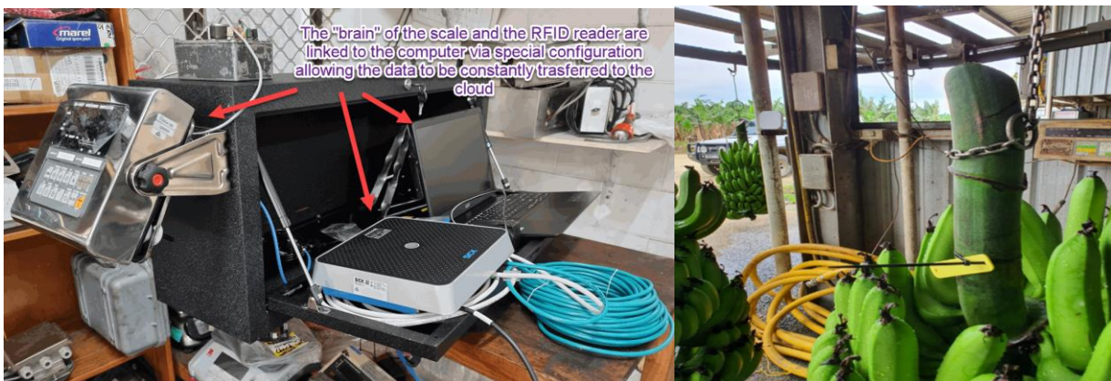
Figure 76. The weight was gathered in the packing shed using an A&D scale. The scale is positioned on the conveyer belt where the banana bunches are hanged.
