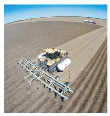
Figure 1 - Anhydrous ammonia 'BIG N' being applied into rows. Photo courtesy of Incitec-Pivot Fertiliser.
