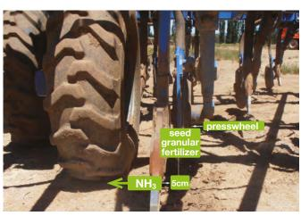
Figure 6 - Front view of the knifepoint for anhydrous ammonia and granular seed/ fertiliser on the application equipment on the commercial vegetable farm in Cowra, NSW.
