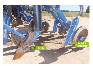
Figure 5 - Side view of the knifepoint for anhydrous ammonia and granular seed/ fertiliser on the application equipment on the commercial vegetable farm in Cowra, NSW.
