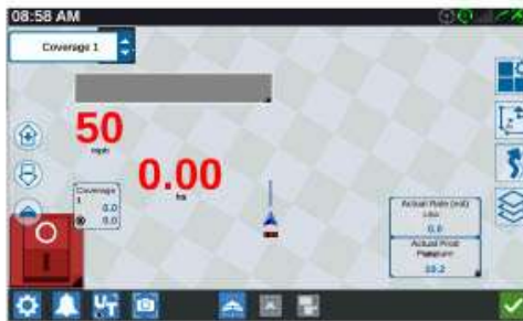
Figure 39: Main switch off
