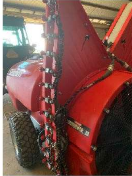
Figure 14: Nozzle wiring harness
