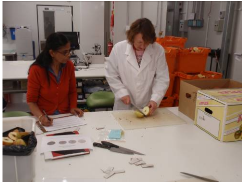
Figure 6 Cutting each fruit in half to assess the level of internal flesh browning.
