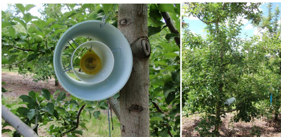
Figure 3 Temperature logger in plastic casing in apple tree.
