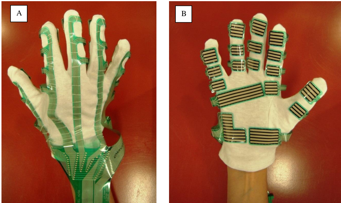
Fig. 2.5 Grip™ e-glove sensor array used to assess shoppers' contribution to flesh bruising of avocado cv. 'Hass' fruit. (A) Top view of the e-glove. Grip™ sensor array sewn onto a white cotton glove with cotton thread. (B) Bottom (palm side) view of the e-glove. After the hand shaped flexible plastic grip sensor platform was sewn to the back of the glove, the grip sensor array pads were folded around the fingers of the cotton glove and attached to the palm side using double-sided tape.
