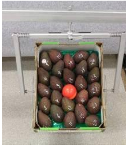
Fig. 2.2 Tray drop setup used for assessment of drop heights and angles effects on bruising in ripening ‘Hass’ avocado fruit.
