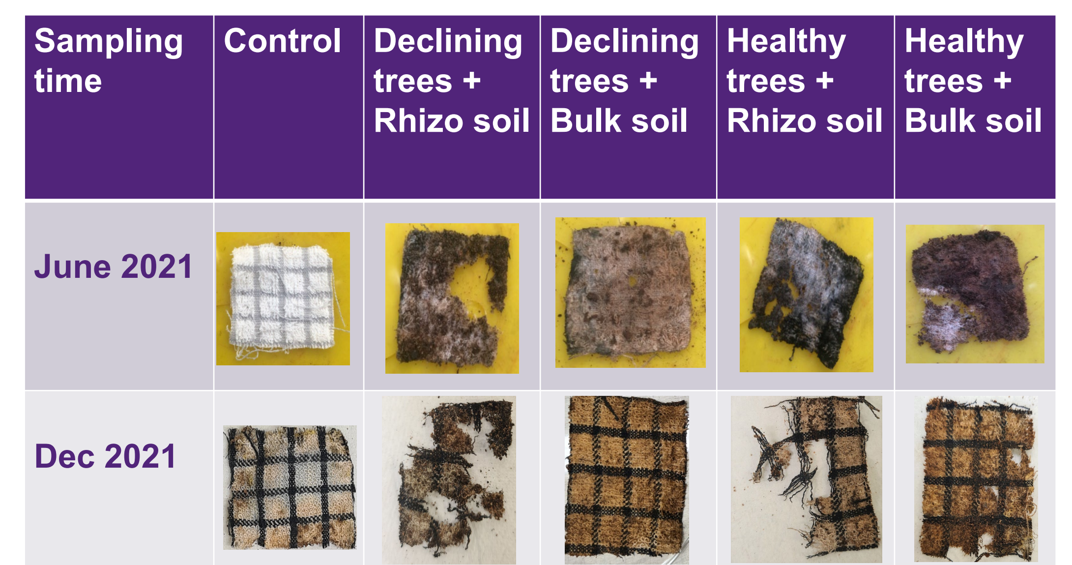
Figure 4. Representative pictures of decomposition of cotton squares after 12 weeks incubation in each soil sample
