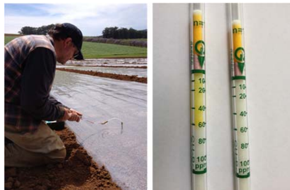
Figure 7: Measuring residues of dazomet and metham sodium in soil using Gastec® tubes.
