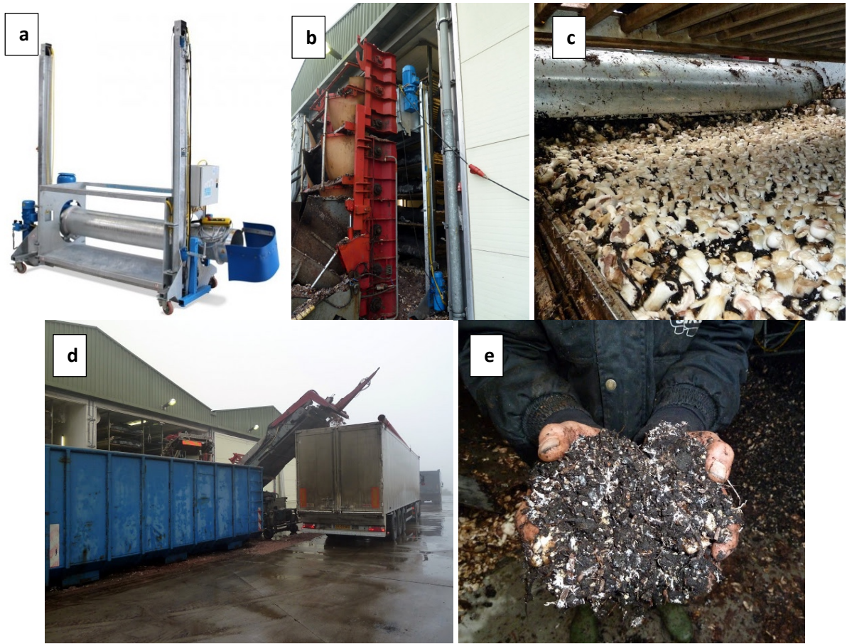
Figure 54. The Mush Comb unit (a) is used to separate the casing from compost during room unloading. The separator is used with a multi-arm emptying machine (b) as the crop is removed after final harvest (c). Conveyors take compost into the waiting trailer, while casing is diverted to a container at one side (d). The separated casing soil (e) and compost can then be recycled or used for other purposes.
