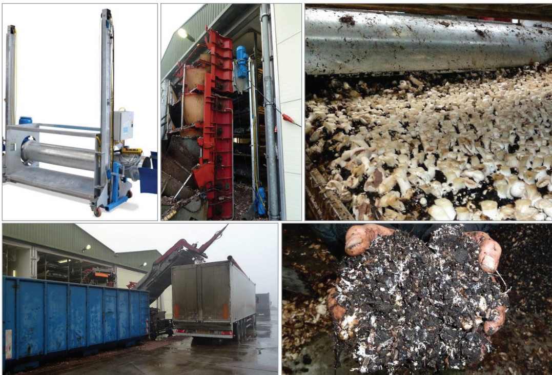
Figure 3. The Mush Comb unit (a) is used to separate the casing from compost during room unloading. The separator is used with a multi-arm emptying machine (b) as the crop is removed after final harvest (c). Conveyors take compost into the waiting trailer, while casing is diverted to a container at one side (d). The separated casing soil (e) and compost can then be recycled or used for other purposes.
