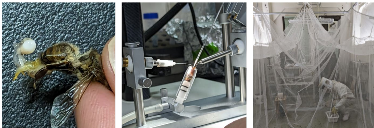
Figure 3: Artificial insemination. (Left) Semen is collected from a drone and (Middle) microinjected into a queen. (Right) Indoor Honey bee colony.
