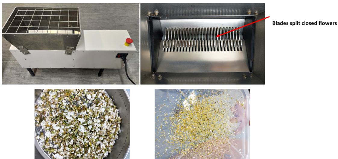
Figure 23. Mill prototype developed in 2020 to split closed flower open to separate the anthers from the rest of the flowers (240 V geared electric motor, 173 rvp, 300 mm x 6 blades, 24 'teeth' on the blade and blade is 3 mm wide).
