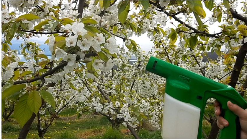
Figure 84. Photo of cordless hand-held electrostatic sprayer (TPSHKE) used to apply pollen
