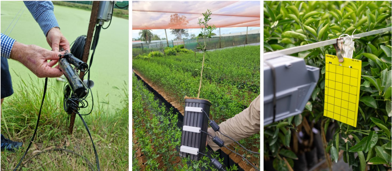
Figure 4. Top three sensors at Golden Grove as rated by the grower. Left to right: Electrical conductivity sensor, soil moisture sensors and pest trap camera
