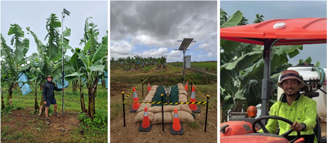
Figure 5. Top three sensors at Bartle Frere Bananas as rated by the grower. Left to right: Soil moisture sensor, nitrate photometer and vehicle trackers
