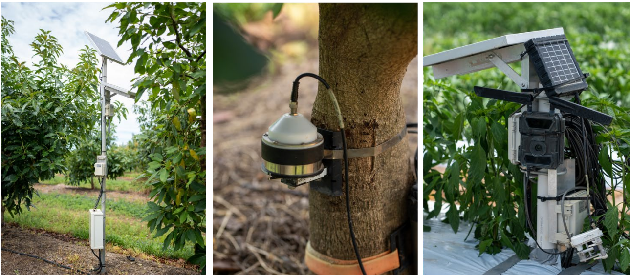
Figure 3. Top three sensors at Austchilli as rated by the grower. Left to right: Soil moisture sensor, band dendrometer and field cameras for growing degree day models
