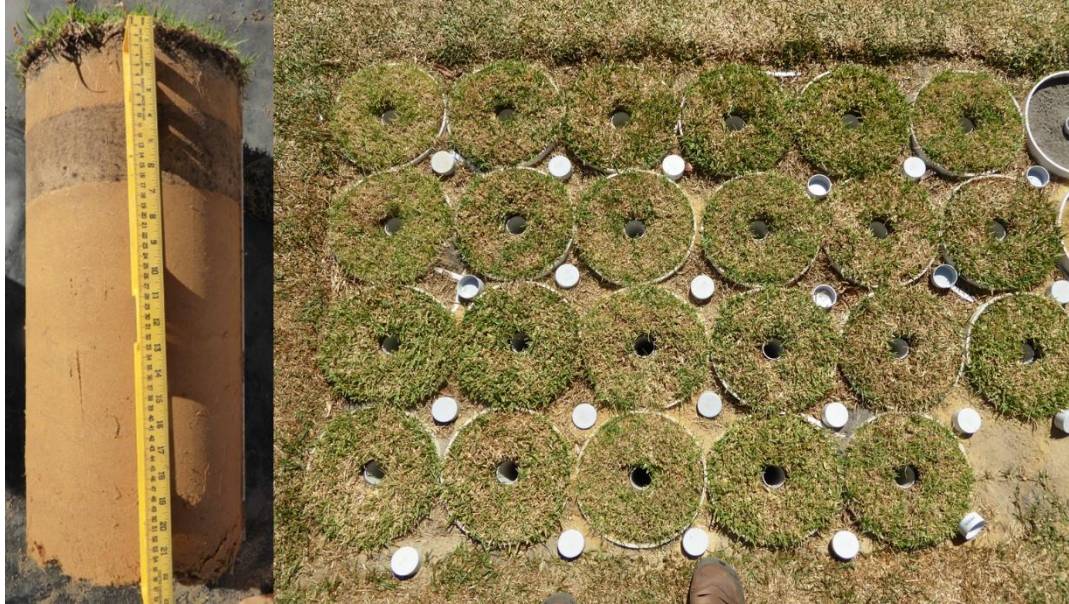
Figure 7. Example of differential turfgrass desiccation during severe drought stress in February 2016 in the soil column experiment (right), and a soil column at the final harvest with compost incorporated in a band at 5-15 cm depth (left).
