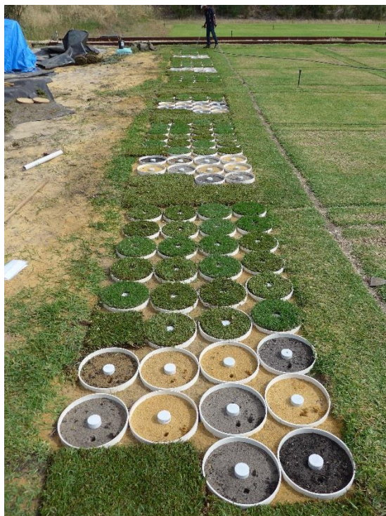
Figure 2. Overview of the soil column experiment to evaluate the effects of incorporating bentonite or compost in a band either at 0-10 or at 5-15 cm depth.
