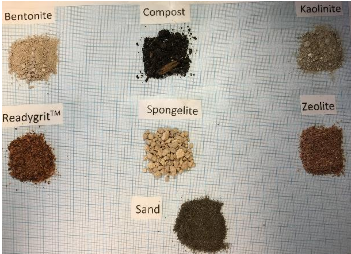
Figure 1. Visualization of applied amendments compared to field site surface sand (top 100 mm).
